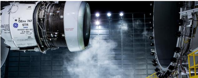
*The GENx engine, shown here after a night of ice testing in subzero temperatures, is embedded with sensors that analyze 5,000 data points every second.*
