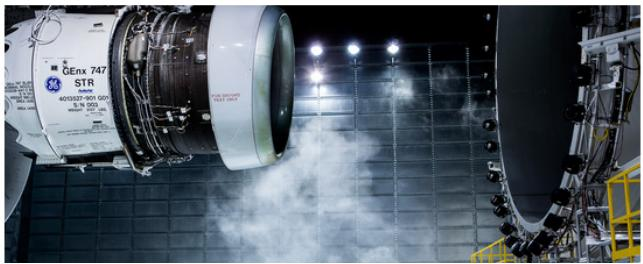
The GEnx engine, shown here after a night of ice testing in subzero temperatures, is embedded with sensors that analyze 5,000 data samples every second.
